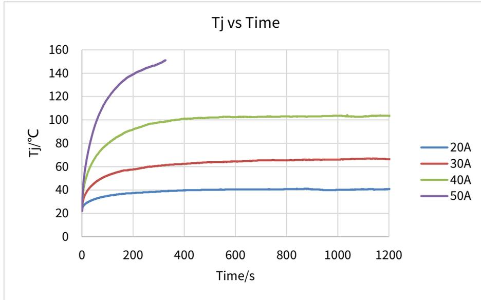
Figure 6.3 NSM2011 Junction temperature vs. Different continues current
